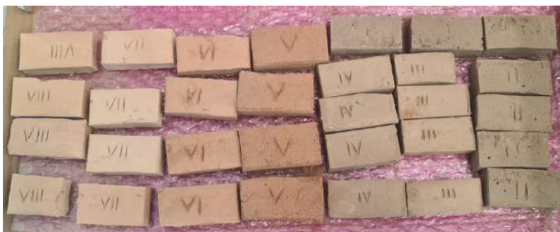
Figure 1: The ready sample product (bricks), made using the samples of the Channel reservoir sediment (Asian Institute for Ecological Research, 2022)
