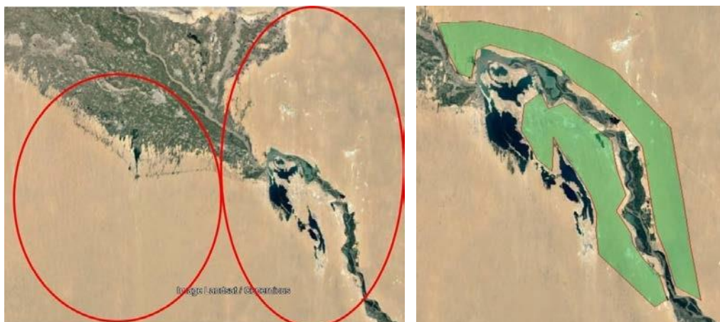
Figure 3-12 Large area around the THC (left image) and along Channel reservoir (right image) to be used for land improvement using removed sediment
