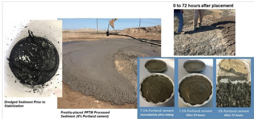
Figure 3-25 Processed sediment using PFTM
