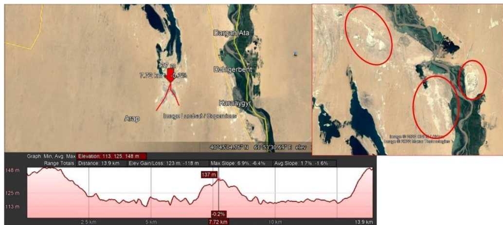
Figure 3-8 Bed profiles along some selected sections of the depressions (based on Google Earth) that could be used as off-channel reservoirs
