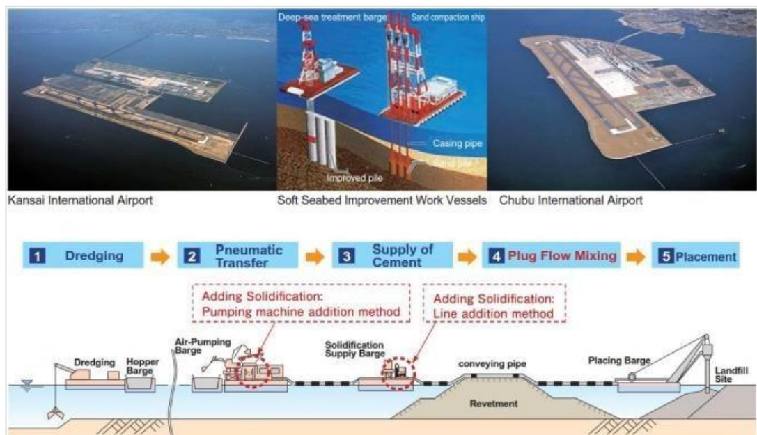
Figure 3-27 Examples of artificial island in Japan (upper images), built using PFTM technique (lower image shows the workflow and features of dredged sediment recycling system (Giri et al., 2019, internet source)
