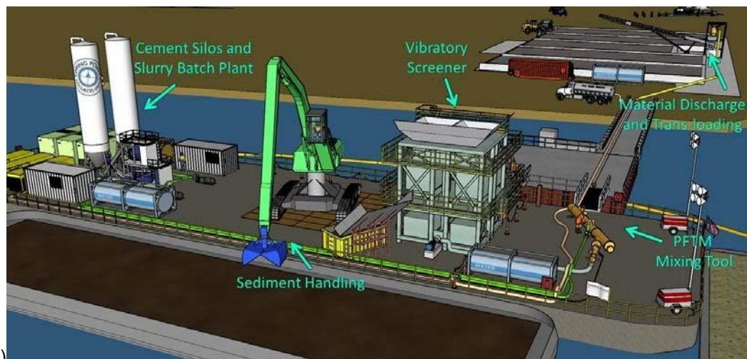
Figure 3-26 Barge-mounted PFTM Operations: Mobile Operating Sediment Engineering System (MOSES)
