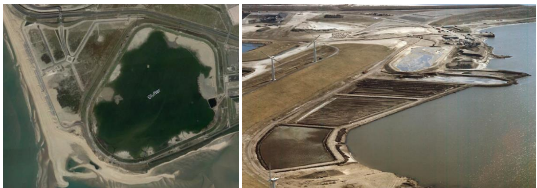
Figure 3-31 A top view of De Slufter (left GE image) and sedimentation basin and clay production fields (right image - Pianc Working Group Envicom 5)
